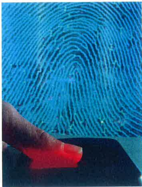
FIGURE 3 Scanning Fingerprints A camera in this scanner takes a picture of a fingertip that is pressed against the glass. The image is stored and viewed on a computer.
