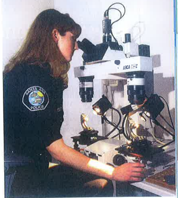
FIGURE 15 Comparison Microscope This microscope is ideal for comparing a sample from a crime scene to a sample from a suspect.
